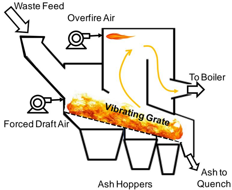
Figure 1. Simplified depiction of a vibrating grate MSW incinerator
