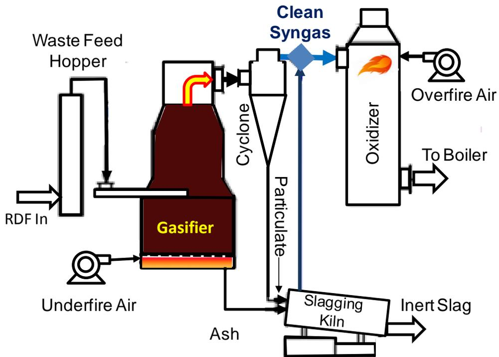
Figure 2. Simplified depiction of an air fed gasification system for the treatment of MSW
